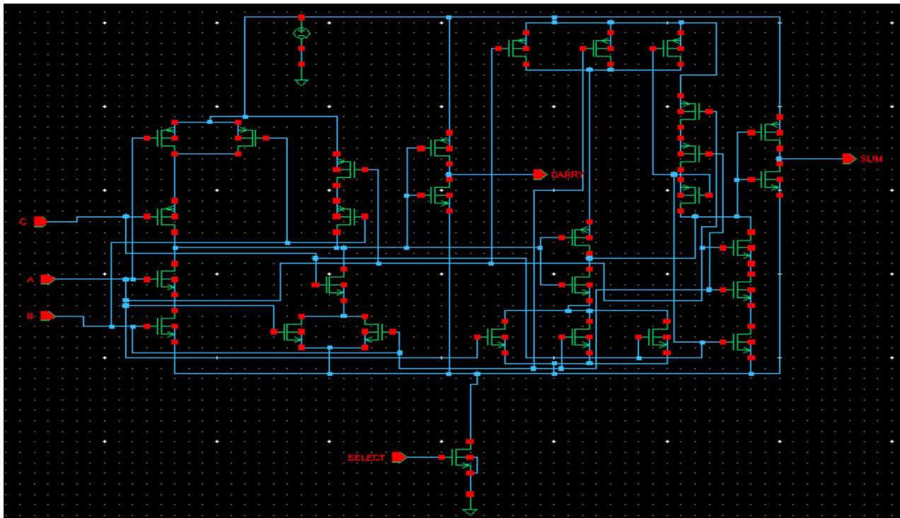
Figure 2: Full adder (Design1) circuit with sleep transistor
