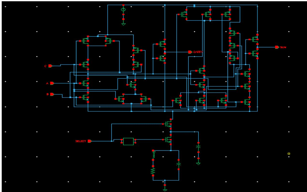
Figure 4: Schematic view of Design 2 with stacking power gating technique (proposed) Modified Design 2
