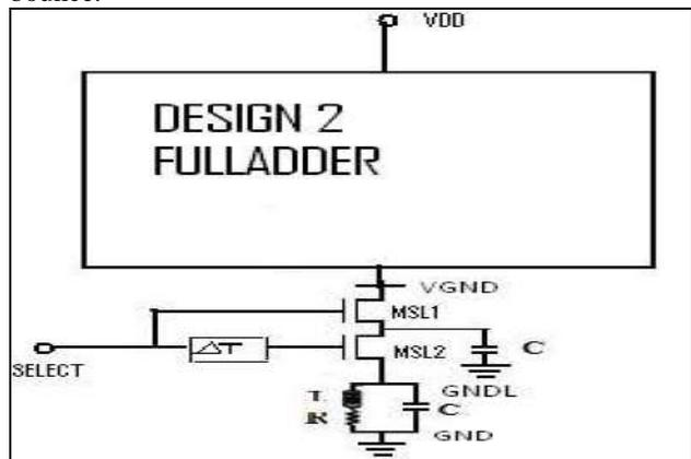
Figure 5: Design 2 with stacking power gating technique (proposed) Modified Design 2
