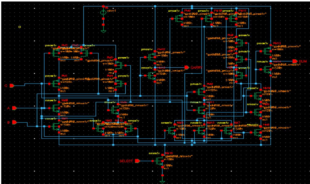
Figure 3: 1 bit full adder (Design2) circuit with sleep transistor
