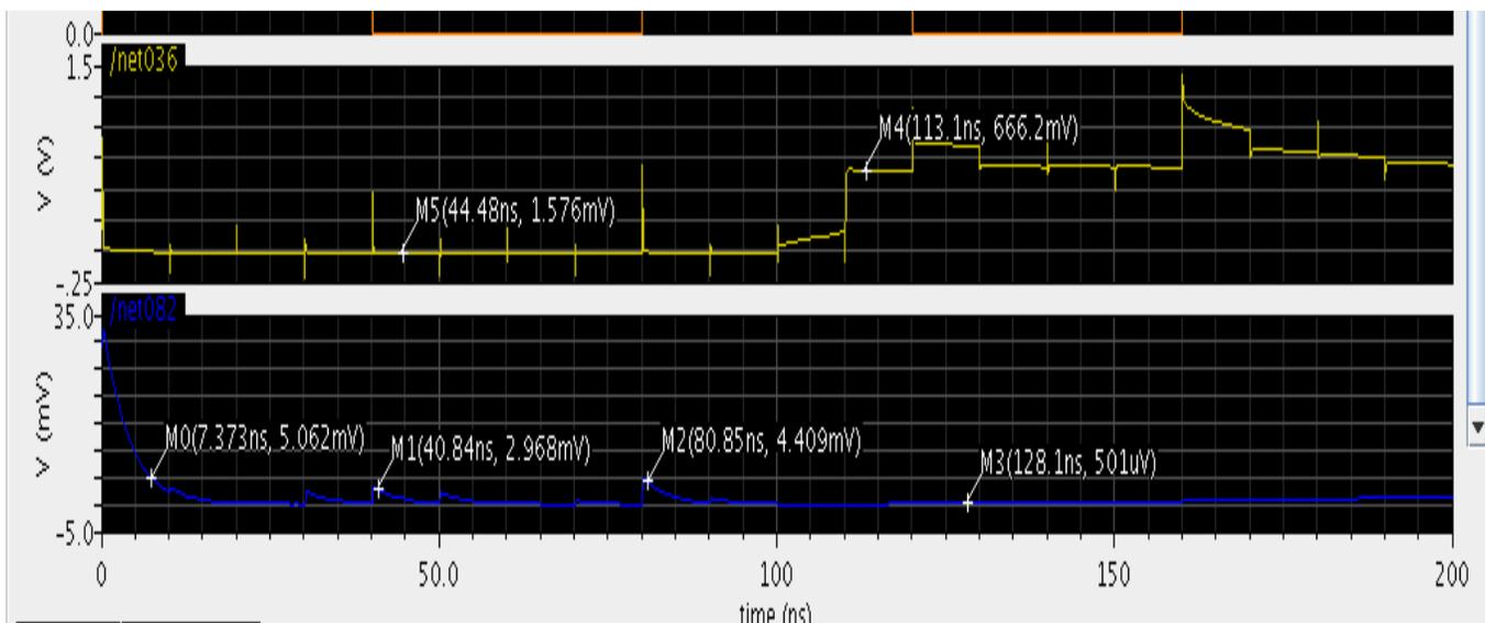
Figure 11: Showing ground bounce noise in design2 with stacking power gating technique without delay
