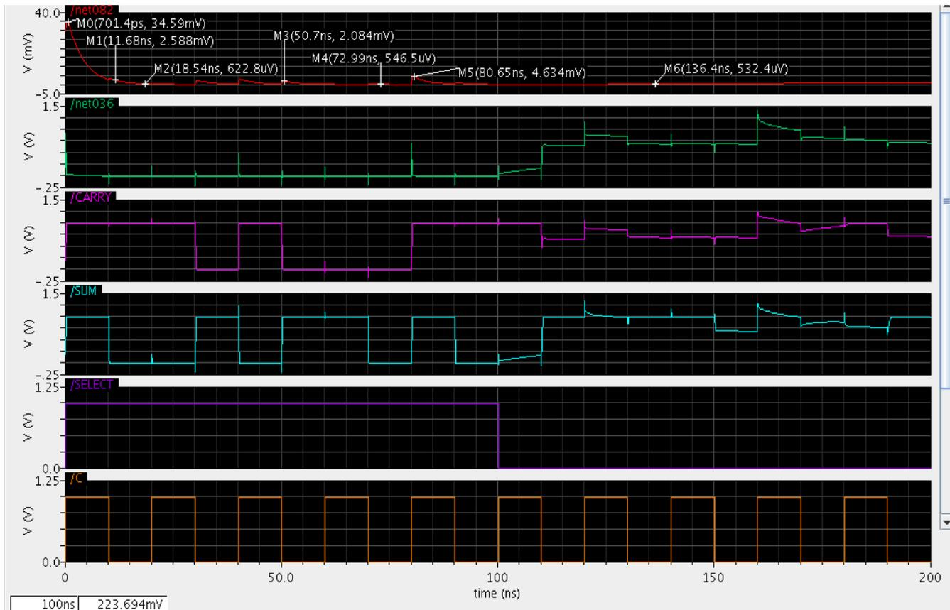
Figure 10: Showing ground bounce noise in design2 with stacking power gating technique with delay
