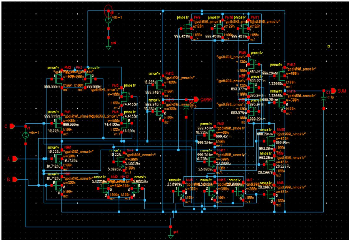
Figure 1: Conventional CMOS full adder.
