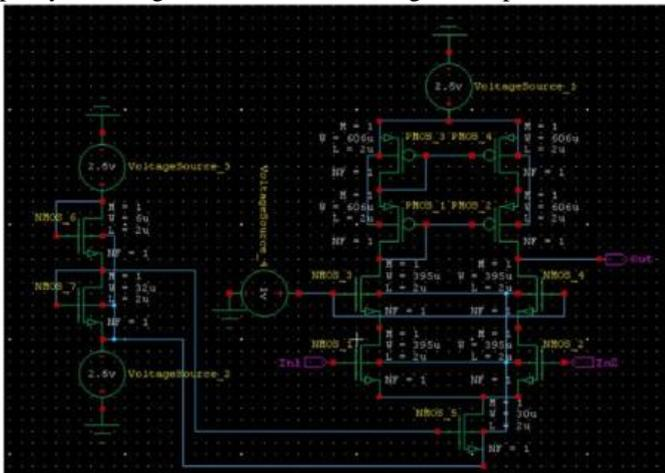
Fig. 3 Circuit implementation of Telescopic OTA
