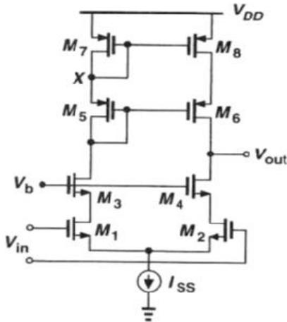
Fig. 2 Circuit diagram of a typical Telescopic OTA
