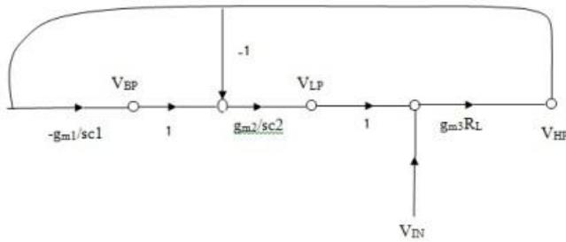
Fig. 7 Signal flow graph of the proposed model
