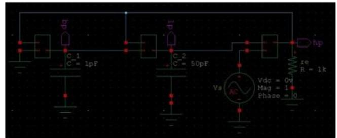
Fig. 6 Simulation model of OTA based KHN filter
