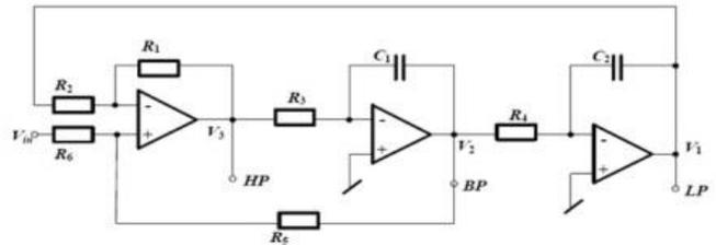
Fig. 5 Typical structure of KHN filter
