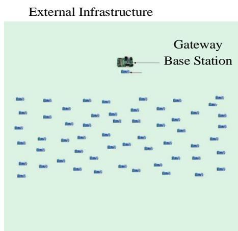
Figure 1. A sensor network with a two-tiered architecture.
