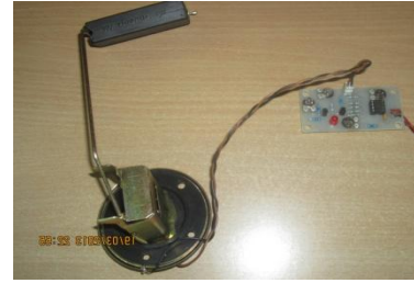
Fig .6 Level Sensor
