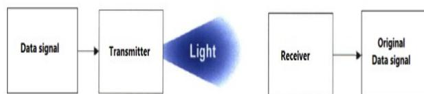
Figure 2.1. Wireless optical communication system overview
