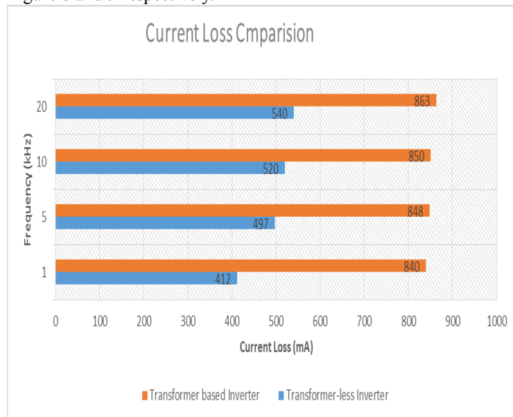
Figure 8: Current loss comparison of transformer-less and transformer based inverter
