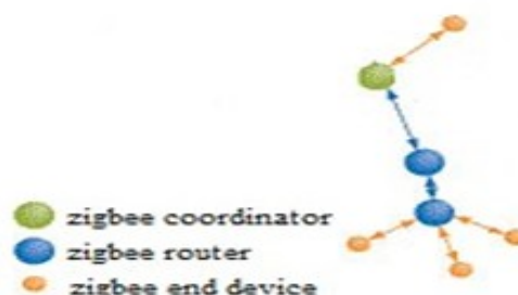
Fig.3 Block diagram of Zigbee based wireless sensor network for the monitoring system
