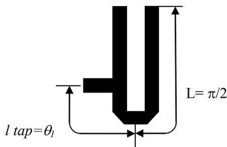
Fig.2 Structure of Tapped Hair pin Resonator
