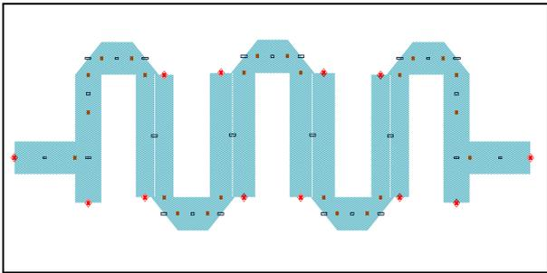
Fig.6. Layout for the 5<sup>th</sup> order Hair pin line BPF
