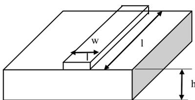
Fig.1 Structure of Microstrip line
