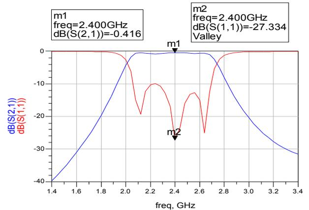
Fig.4 Simulated results (Reflection & Transmission coefficients) of BPF
