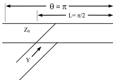
Fig.3 Equivalent of Tapped Hair pin Resonator
