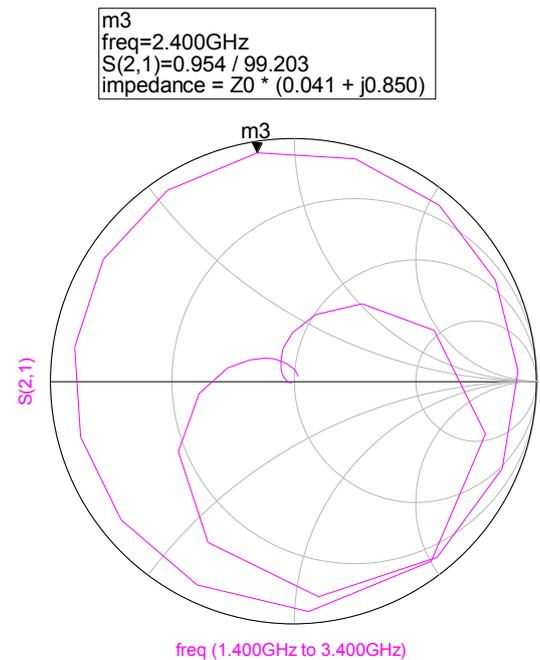
Fig.5 Simulated results (Reflection coefficient) of BPF in Smith chart
