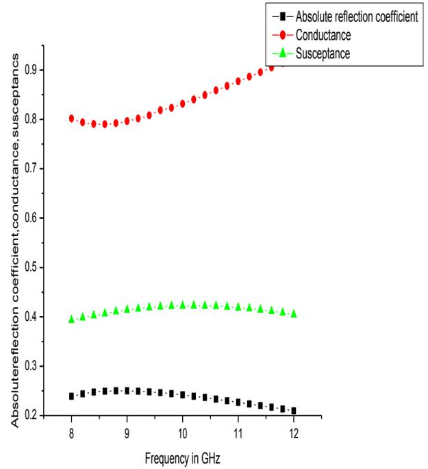
Fig.7 Absolute reflection coefficient, radiation conductance and susceptance for single radiator
