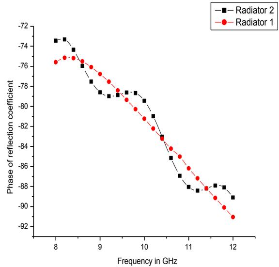
Fig.3 Phase of the Reflection coefficient for the radiating array element
