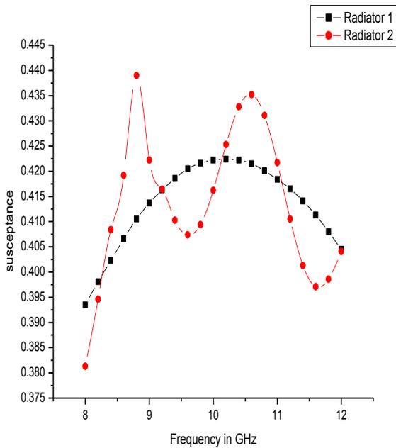
Fig.6 Radiation susceptance for array elements
