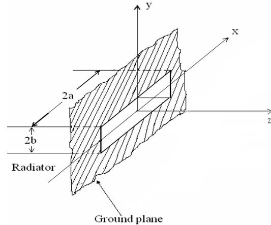
Fig. 1 Schematic diagram of open ended waveguide radiator.
