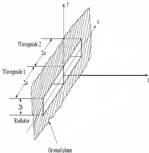
Fig. 2 Schematic diagram of open ended waveguide of two element array radiator.
