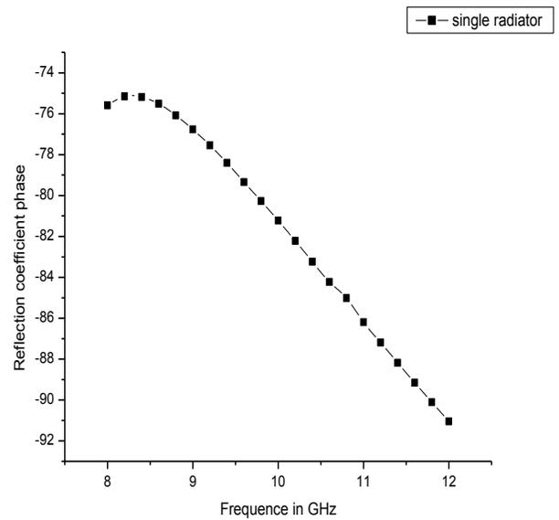
Fig. 8 Reflection Coefficient Phase, for single radiator
