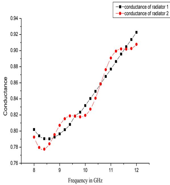
Fig.5 Radiation conductance for array elements
