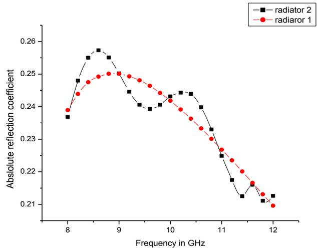
Fig.4 Reflection coefficient (absolute) for the radiating array element
