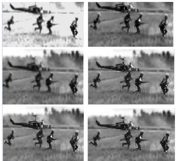
Fig 7. Fused images obtained using averaging, select maximum, PCA, DCT, DWT, SWT respectively (in sequence starting from left most image)
