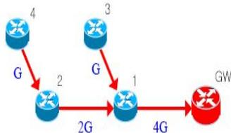
Figure 9: Multi-hop Wireless Network with four nodes and single gateway
