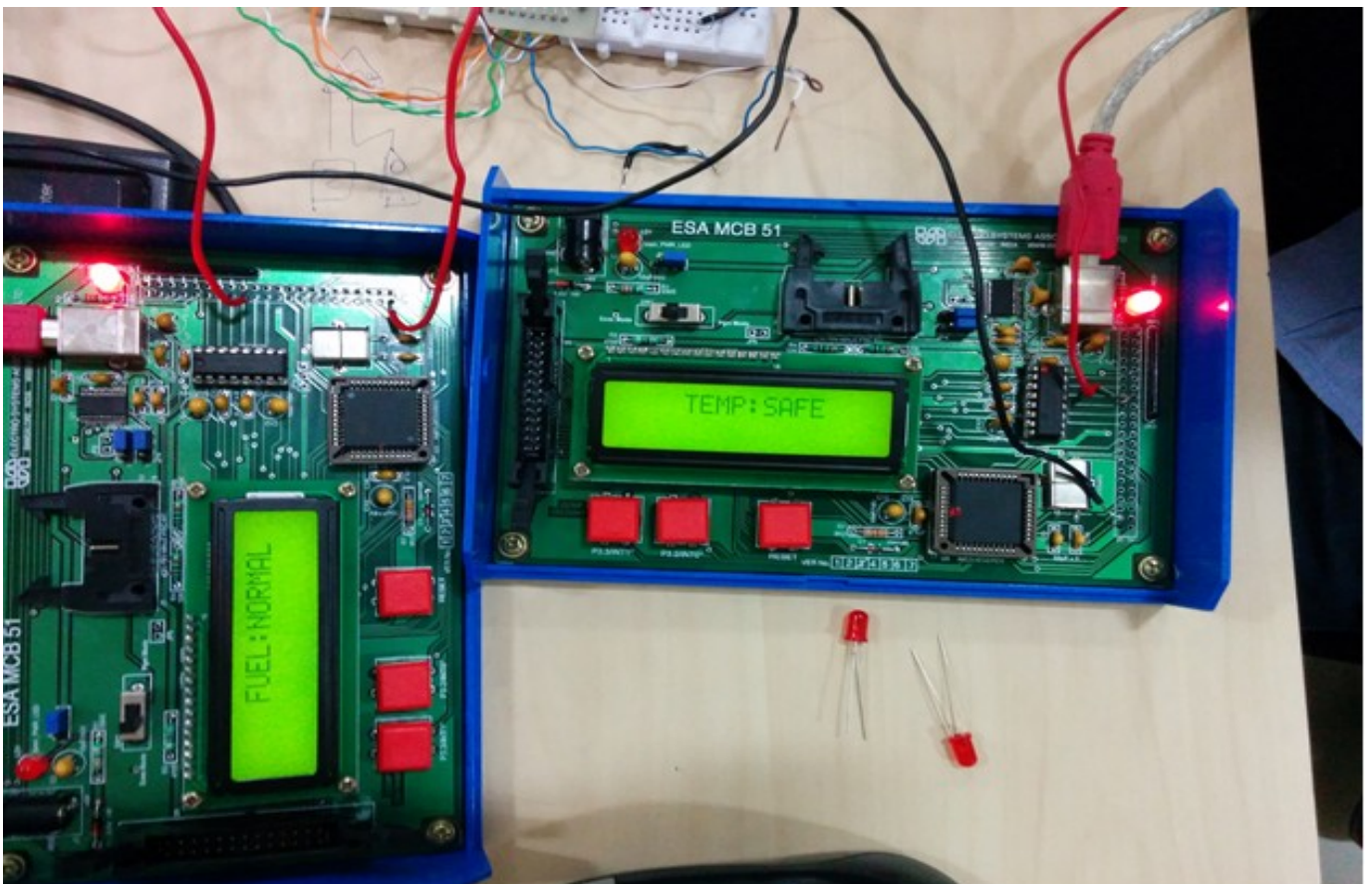
Fig 7: LCD Display and temperature LEDs
