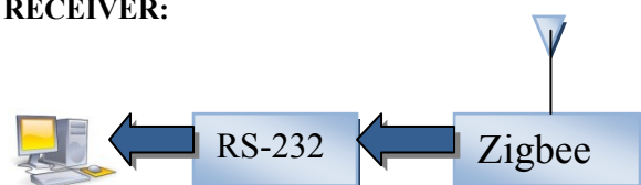
Fig. 2 Block Diagram of Receiver
