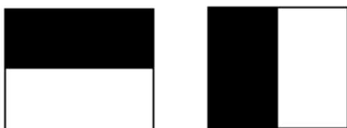
Fig 6: Haar-wavelet response in x and y direction [2]
