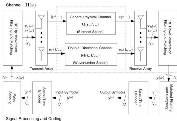
Fig 3: Block diagram of a generic Multiple-Input Multiple-Output wireless system
