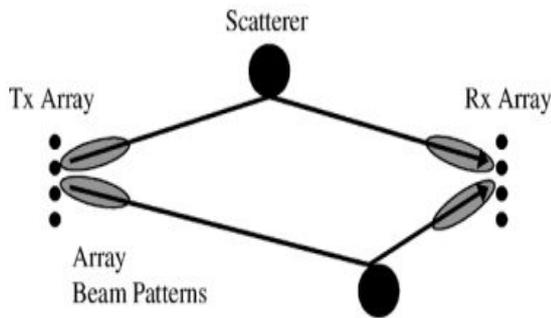
Fig 2: Simple Multipath Propagation Environment
