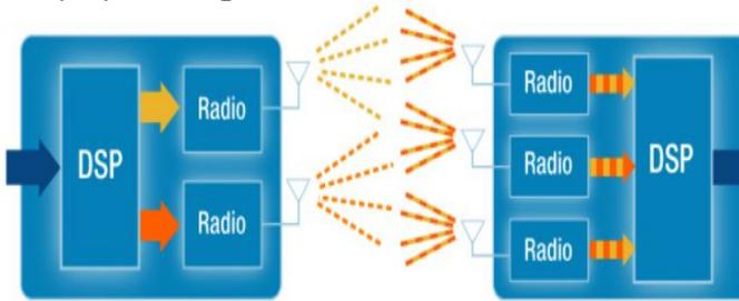
**Fig 7: MIMO Signals from Transmitters to Receiver**
