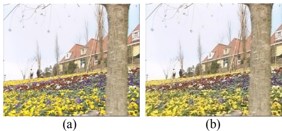
Figure 4: (a) Original 2 nd Frame of flower sequence (b) Marked frame with DWT, PSNR=28.25
