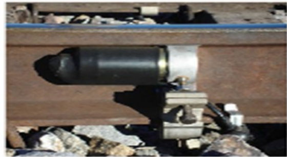
Fig.1 Ultrasonic Broken Rail Detector
