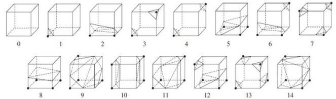
Figure 2: Cube-Isosurface Intersection Patterns
