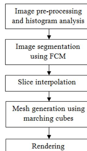
Fig 1: flowchart for 3D reconstruction.
