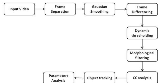
Figure1: Block diagram.
