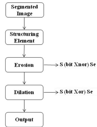
S – Segmented Image, Se = 'disk' Structuring Element
