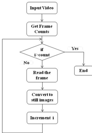
Figure2: Process flow.
