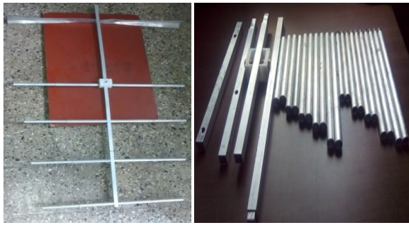
Fig. 5 Fabricated Yagi-Uda Antenna and its portable form
