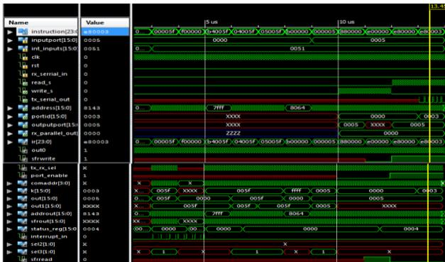
Fig. 7. Simulation results for Interrupt controller, transmitter and RISCPU
