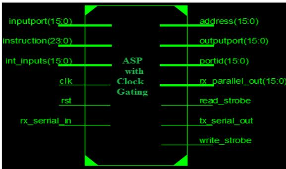
Fig. 2. Signals of ASP with Clock Gating Technique
