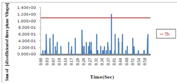
Fig.6.h.Sum of absolute magnitude of detailed coefficient d1 of three phase voltages under B phase turn fault
