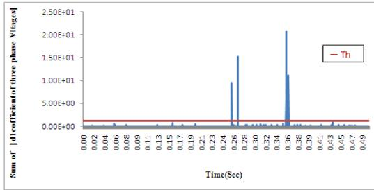
Fig.6.f.Sum of absolute magnitude of detailed coefficient d1 of three phase voltages
