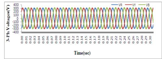
Fig.6.a. Three phase normal voltages of 3-ph induction motor
