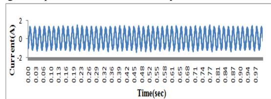
Fig.4.b.Y phase current under healthy condition
