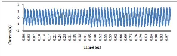
Fig .5.a.Variation of R phase current under R phase turn fault on 3-phase induction motor.
