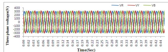
Fig.6.c. Variation of 3-ph voltages under R phase turn fault on 3-phase induction motor.
