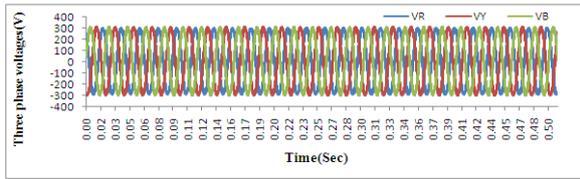
Fig.6.e.Variation of 3-ph voltages under Y phase turn fault on 3-phase induction motor.
