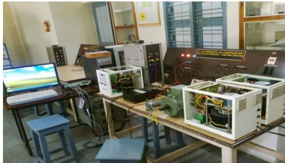
Fig .3.a.Experimental set up of three phase Induction motor Stator inter turn fault detection.
