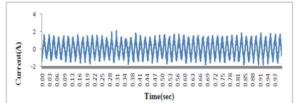
Fig .5.c.Variation of B phase current under B phase turn fault on 3-phase induction motor.
