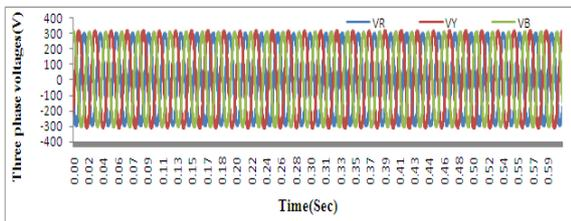
Fig.6.g.Variation of 3-ph voltages under B phase turn fault on3-phase induction motor.
