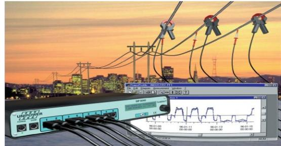
Fig .3.b.Power network analyzer
