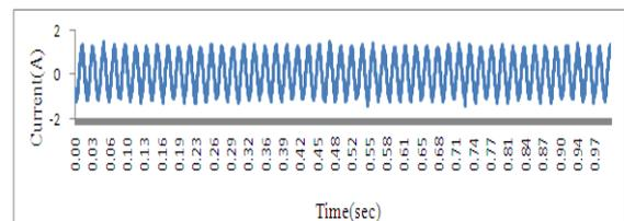
Fig.4.c.B phase current under healthy condition
