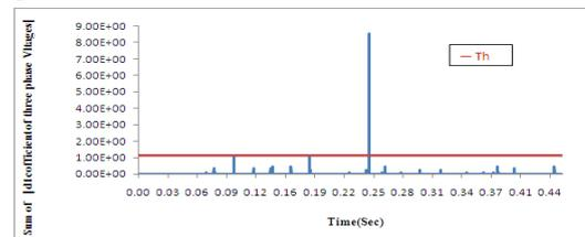
Fig.6.d. Sum of absolute magnitude of detailed coefficient d1 of 3-ph voltages under R phase turn fault
