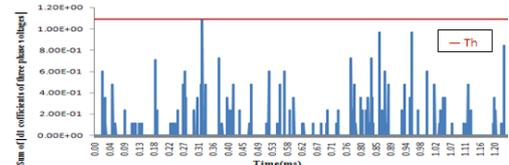
Fig.6.b.Sum of the absolute value of the detailed coefficient d1 of three phase voltages
