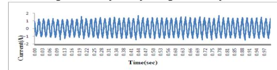
Fig .5.b.Variation of Y phase current under Y phase turn fault on 3-phase induction motor.
