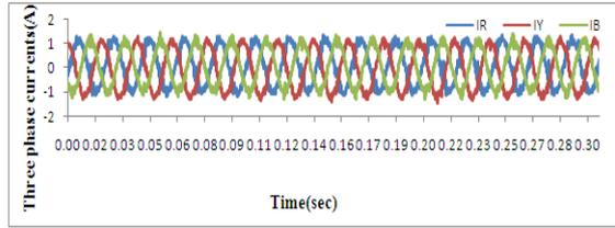
Fig.5.d. Normal three phase currents of 3-ph induction motor
