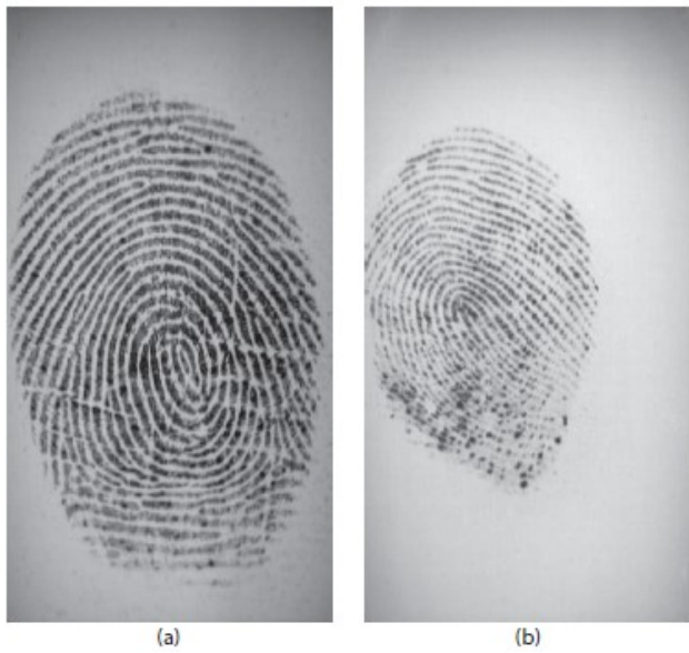
Fig 1:Fingerprint sensor images of the (a) little finger of a 30-year-old man, and the (b) little finger of a 5-year-old boy, illustrate the varying fingerprint image quality.
