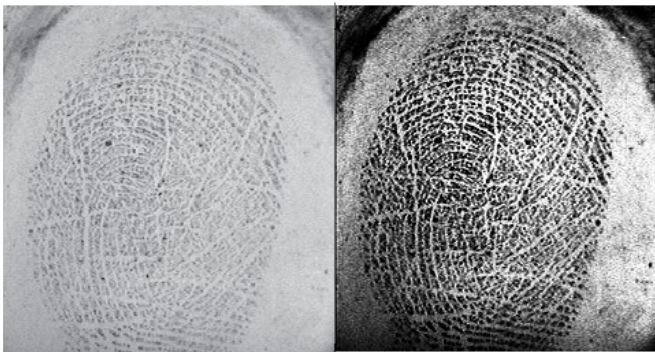
Fig4: original image (left) and after histogram equalization (right)
