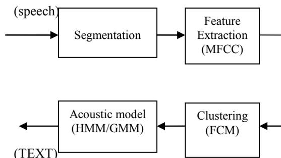
Fig 1:Block Diagram of CSR system
