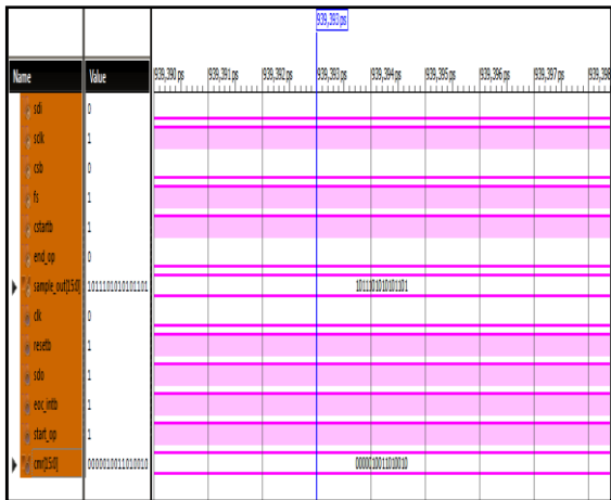
Fig 5. Simulation of TLC2578 ADC
