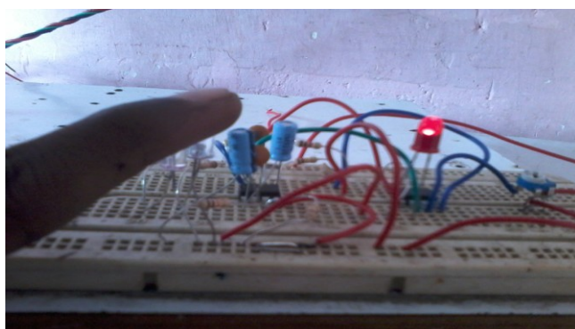
Fig.4. Bread Board Simulation of Heart Rate Sensor
