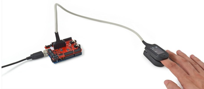
Figure 6: Pulse Oximeter Data Acquisition using Intel Galileo and e-sensor shield
