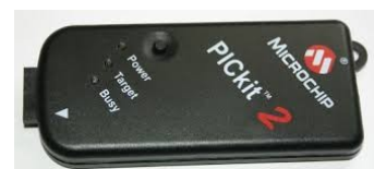
Fig 6: PIC kit 2 for downloading hex file
