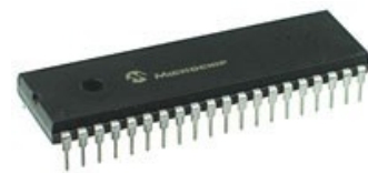
Fig 2: PIC18F4520 Microcontroller in PDIP Package
