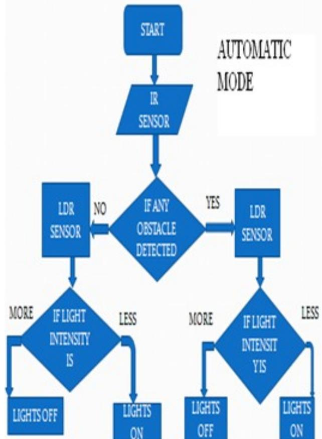
Fig.5 Flow Chart for auto mode operation
