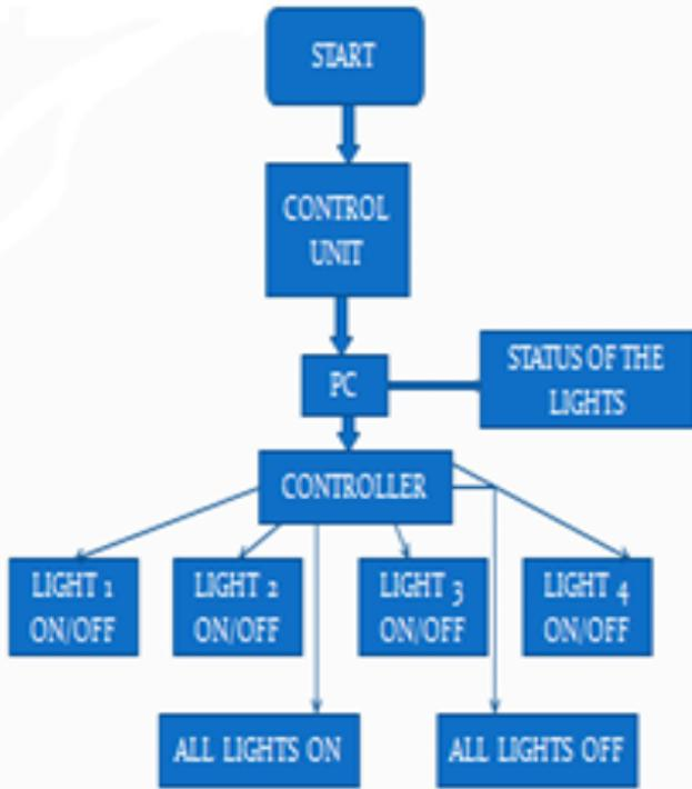
Fig.6 Flow Chart for manual mode operation
