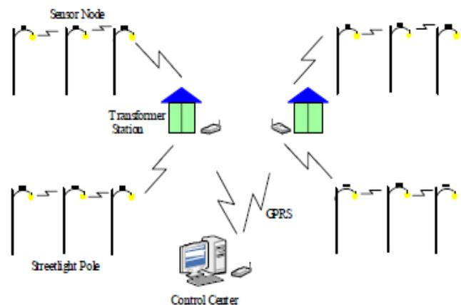
Fig.3 Structure of streetlight power cable monitoring system based on wireless sensor networks
