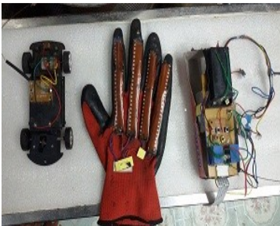
Figure: 4 Experimental setup of flex sensor
