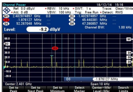
Fig. 12. Spectrums showing Channel Power for the data being transferred using SPP Application
