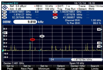
Fig. 11. Spectrums showing occupied Bandwidth for the data being transferred using SPP Application
