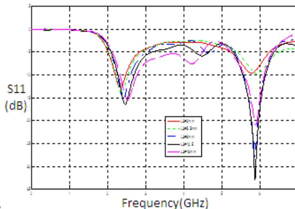
Fig. 3. (C) The variation of L3 parameter on the return loss.
