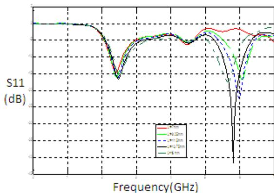
Fig. 3. (A) the variation of L1 parameter on the return loss.
