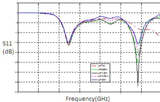
Fig. 3. (D) The variation of L4 parameter on the return loss.
