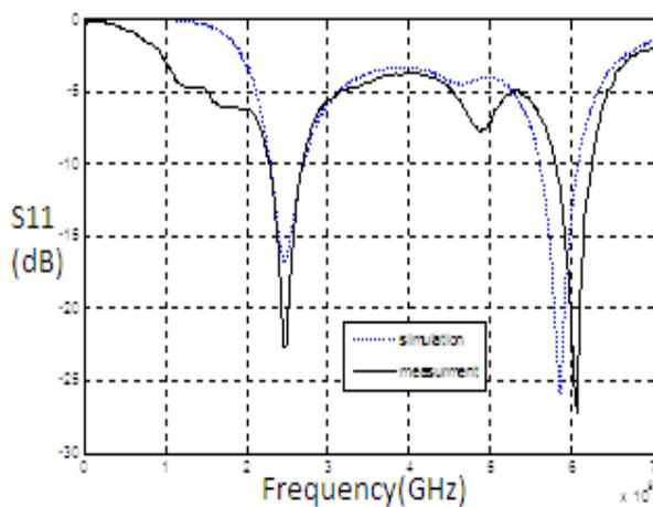
Fig. 4: S11 simulated and measured return losses of proposed antenna.
