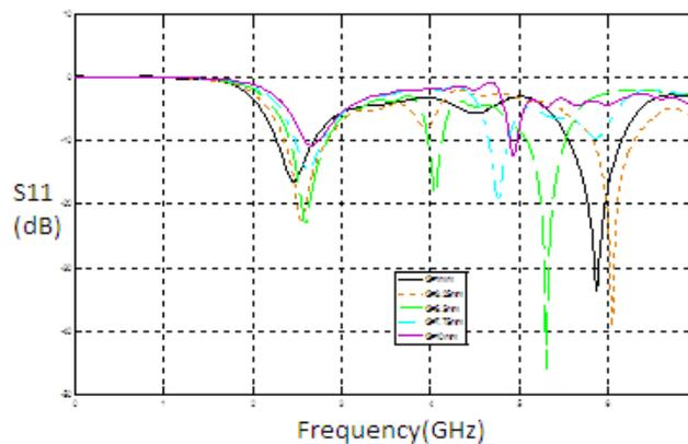
Fig. 3. (E) The variation of Ground (G) parameter on the return loss.
