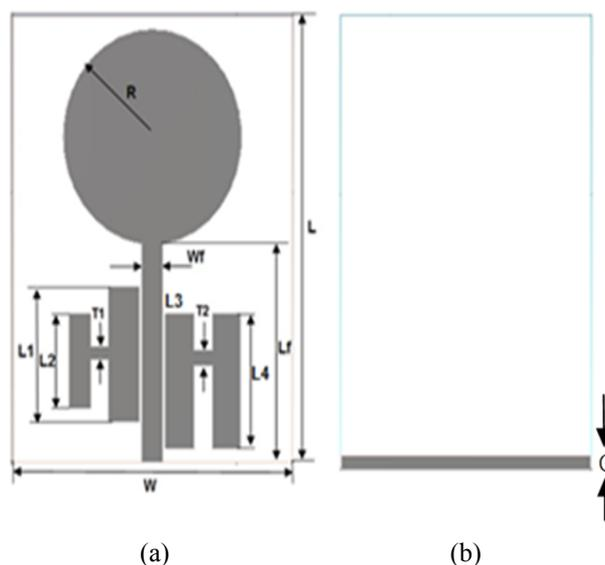
Fig.2: Antenna geometry structure (a) Top view, and (b) Bottom view.
