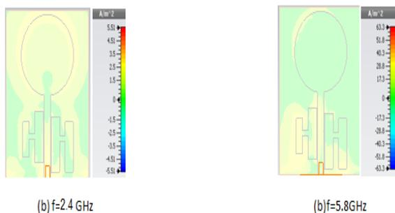
Fig. 8. simulated current distribution at different frequencies(2.4 GHz & 5.8 GHz)
