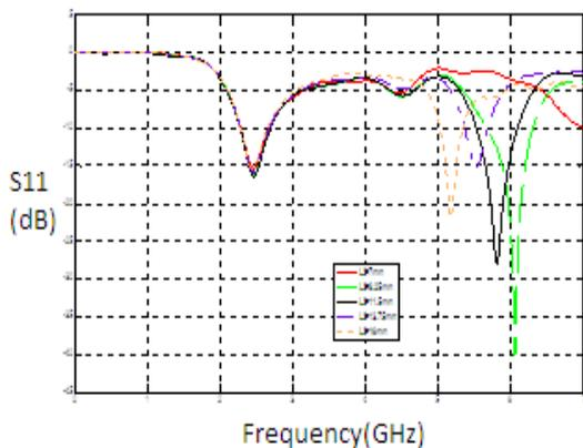
Fig. 3. (B) the variation of L2 parameter on the return loss.
