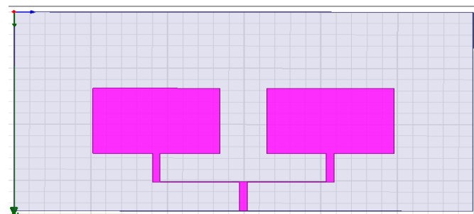
Fig 4. Simulated diagram of Rectangular array micro strip patch antenna
