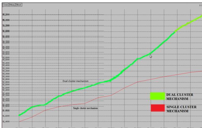
Figure 7 Comparison graph of Single and Dual cluster mechanisms for Packet delivery ratio
