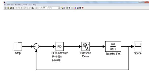
Figure 5.3 Simulink Model for Skogestad Method
