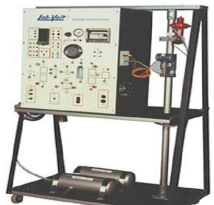
Figure 4.1 Pressure Process Training System
