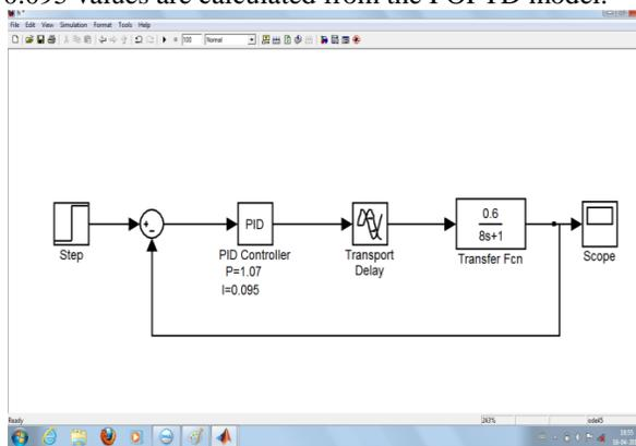
Figure 5.1 Simulink Model for Cohen Coon Method
