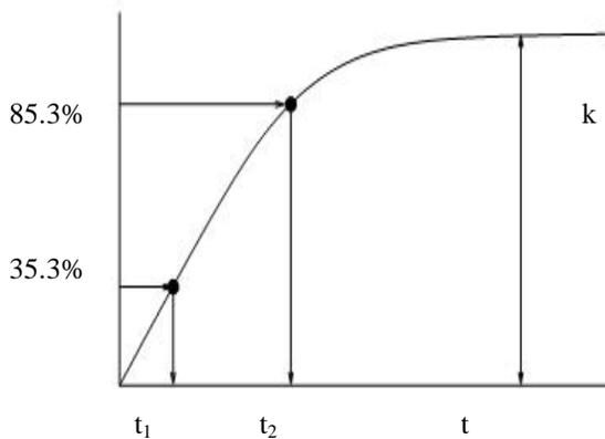
Figure 2.1 Time Vs System Response graph
