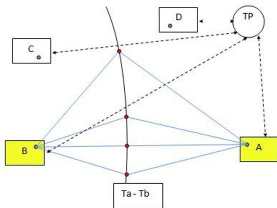
To get a two dimensional point, three RUs are required. 3 RUs develop intersecting hyperbola, 2D formula is used (no Z axis). 2d position is generated
