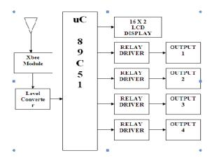
In receiver, all these wireless data received by the receiver. This is given to the microcontroller through the level converter IC max 232. Xbee operates on 232 and microcontroller operates on TTL. They are not compatible so we used level converter. This signal is goes to microcontroller.
