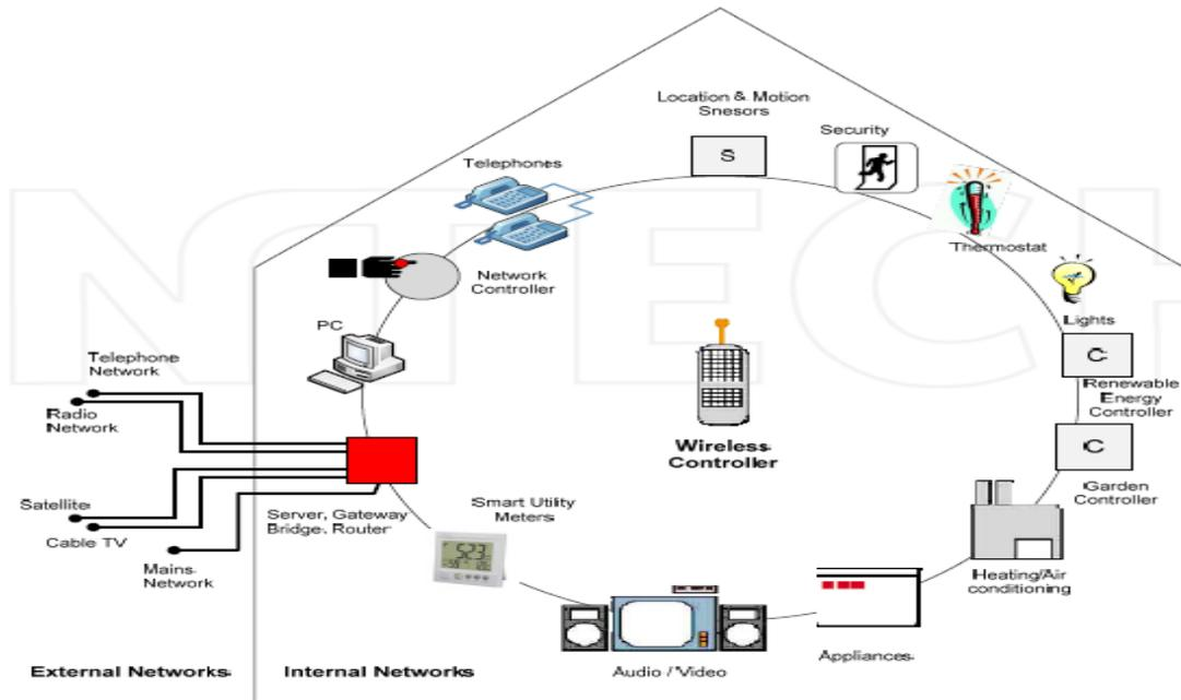
Fig. 1. Basic smart home network system architecture [7].
