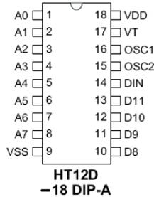
Fig 4.4 Pin Diagram of HT12D decoder
