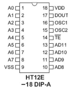
Fig 4.3 Pin Diagram of HT12E encoder
