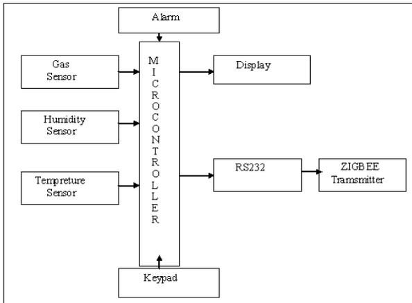
Fig.1 Transmitter system
