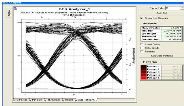
Figure 10: Eye diagram analysis for 2<sup>nd</sup> Channel of Symmetrical Compensation Technique at 1550nm Wavelength
