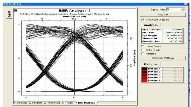
Figure 7: Eye diagram analysis for 2<sup>nd</sup> Channel of Post Compensation Technique at 1550nm Wavelength
