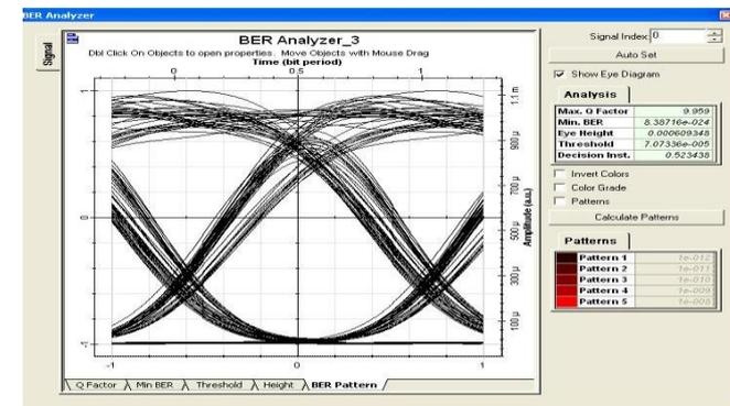
Figure 5: Eye diagram analysis for 4<sup>th</sup> Channel of Pre Compensation Technique at 1550nm Wavelength
