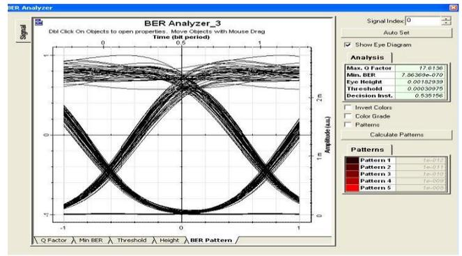
Figure 9: Eye diagram analysis for 4<sup>th</sup> Channel of Symmetrical Compensation Technique at 1550nm Wavelength
