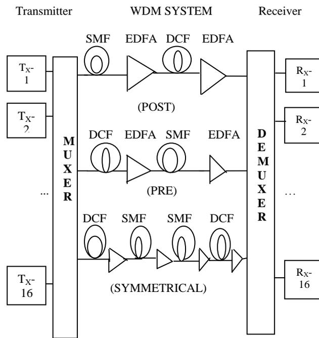
Figure 2: Optimized Link for 16-Channels WDM system using dispersion compensating fiber technique (Pre, Post, and Symmetrical Compensation)
