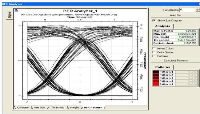
Figure 4: Eye diagram analysis for Second Channel of Pre Compensation Technique at 1550nm Wavelength
