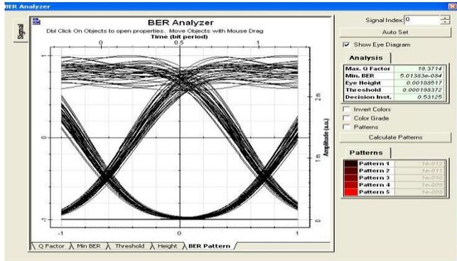
Figure 9: Eye diagram analysis for first Channel of Symmetrical Compensation Technique at 1550nm Wavelength
