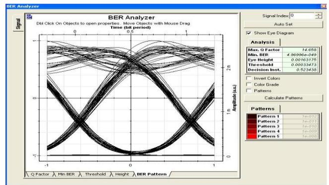
Figure 6: Eye diagram analysis for 1<sup>st</sup> Channel of Post Compensation Technique at 1550nm Wavelength
