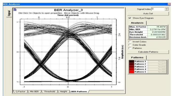
Figure 8: Eye diagram analysis for 4<sup>th</sup> Channel of Post Compensation Technique at 1550nm Wavelength
