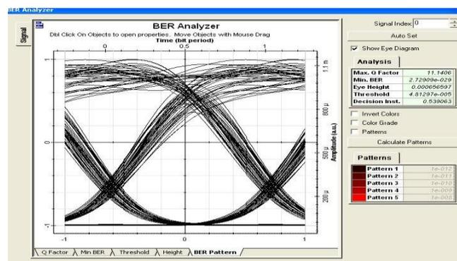
Figure 3: Eye diagram analysis for first Channel of Pre Compensation Technique at 1550nm Wavelength
