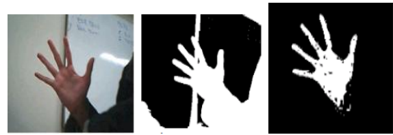
Figure 2-2. Conversion of RGB colors into gray scales and YCrCb for binary representation
