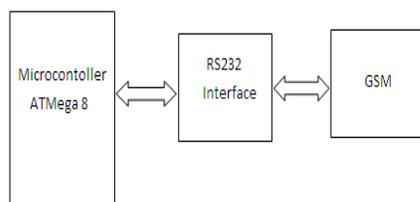
**Fig. 6 GSM modem**
