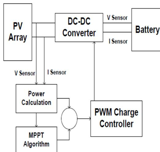
**Fig. 5 Block diagram of MPPT Charge Controller**
