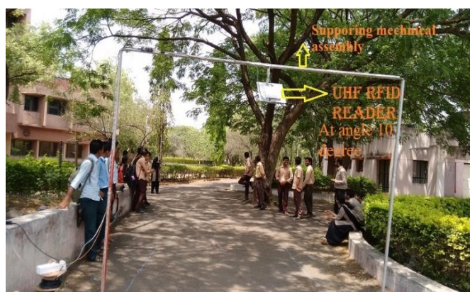
Fig 3: System Setup at Normal check point front view (Reader tilted at 10° with Horizontal Plane)
