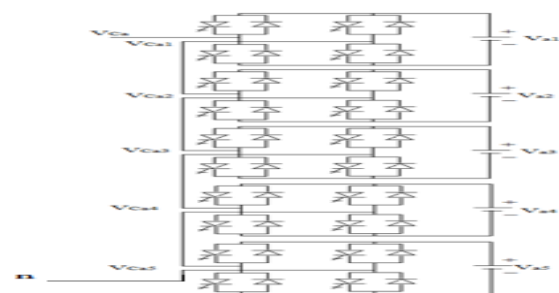
Fig. 4 Single-phase 11-level cascaded inverter
