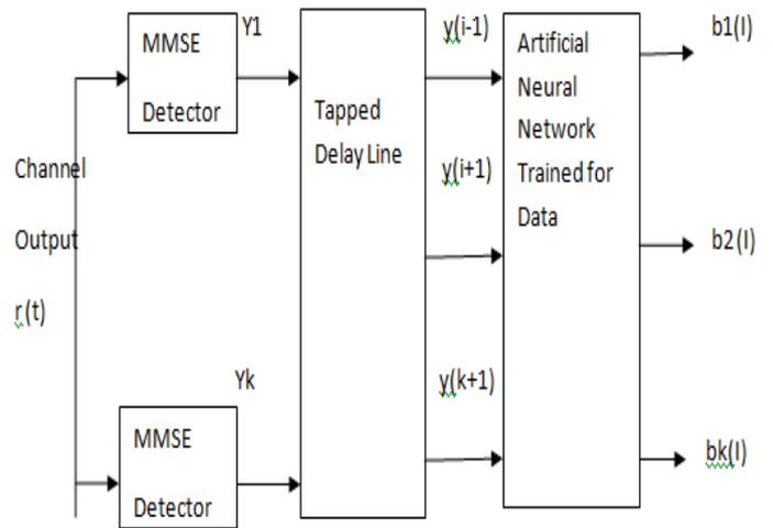
FIG (4)–MMSE Detector with Artificial Neural Network (ANN).
