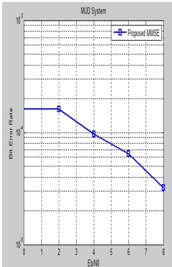
FIG(6) - BER and SNR of Proposed MMSE
