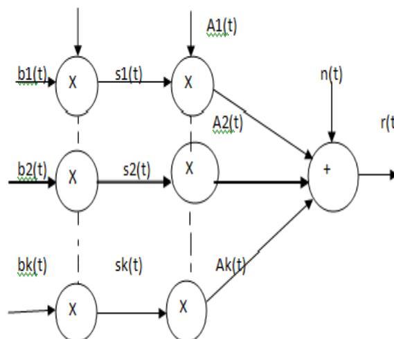
FIG (1) - System model for DS-SS System
