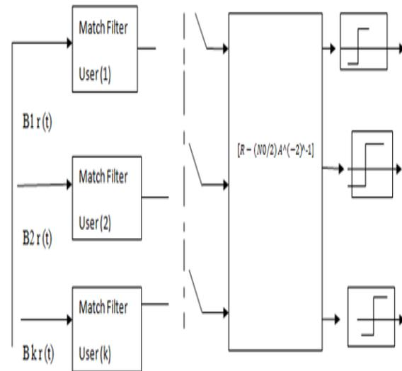
Fig (2) – MMSE Detector with Matched Filter
