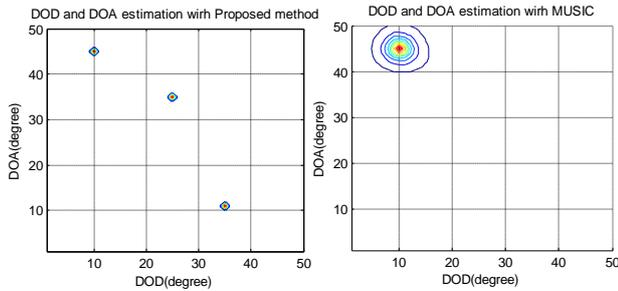
Figure 2.comparison of our method with RD-MUSIC for bistatic MIMO radar with coherent targets
