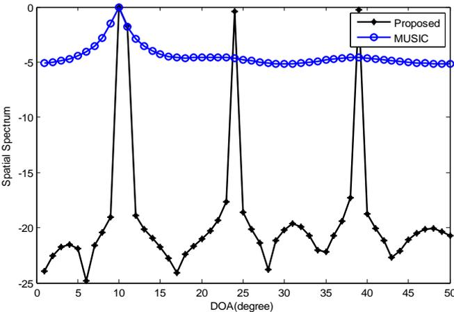
Figure 3.comparison of our method with RD-MUSIC for mono-static MIMO radar with coherent targets
