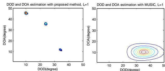
Figure 1. Comparison of our method with RD-MUSIC for bistatic MIMO radar with non-coherent targets.
