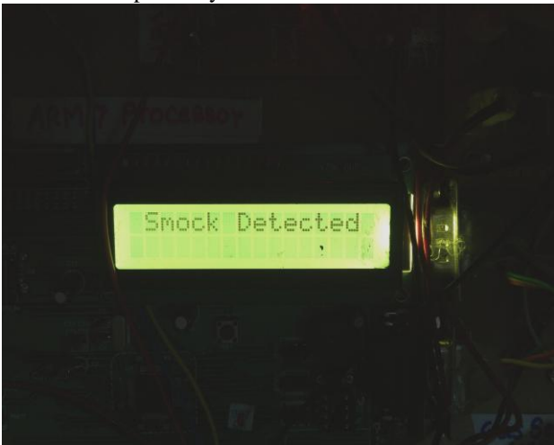
Fig 4.2 When gas values increases above its threshold value
