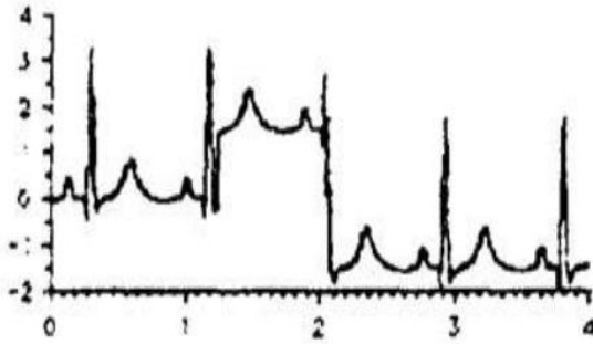
Fig. 1 ECG corrupted due to abrupt Baseline Drift
