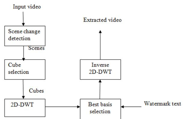
Fig.3 Block diagram of video watermarking using best basis selection
